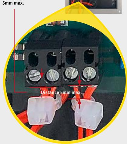
**Note:** When connecting the telephone line or additional power supply, note the position of the two cable ties (included in the box)
