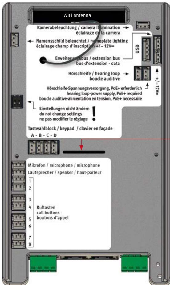
For 20-0003-BS, 20-0015-BS, 20-0017-BS, the connection cable for the Behnke touch display is located here
